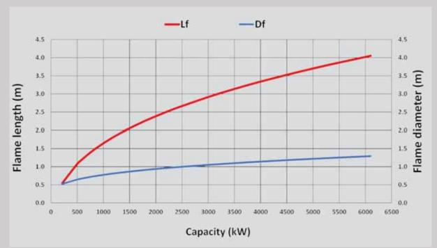
The flame dimensions which play an effective role in the burner efficiency and influence their compatibility to the boiler combustion chamber geometry, are presented in the above diagram.
