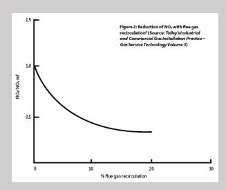
When FGR is used, because of reduction in radiation heat transfer, boiler efficiency may decrease, typically in the range of 0.25 percent to 1 percent, depending on the amount of FGR added. Plant experience shows that the combination of low NOx burners with re-burning using FGR system, reduces the NOx level to approximately lower than 40 mg/kWh.
