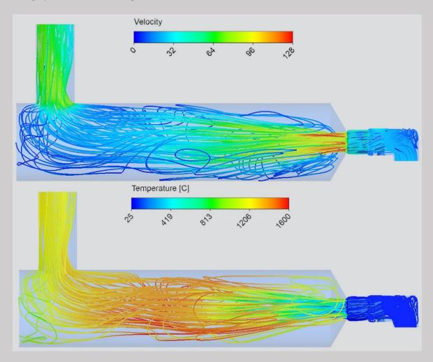
Heat generators with very high medium temperatures can exploit less of the heat in the flue gases. Consequently, flue gas temperatures are always higher than the medium temperature. Without additional heat exchangers, a lot of energy will be lost to the atmosphere and wasted. One way of utilizing this energy is through the use of hot-air versions of the DB-series dual-bloc burners.
