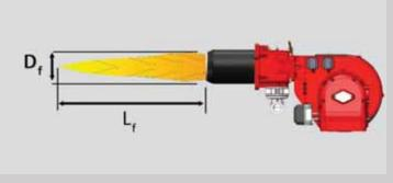
BS-2790, BS-855, EN-303, BS-EN 12953-3. It is recommended that a flame fill 90% of combustion chambers at its maximum output.
