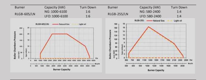
Working diagrams for light fuel oil burner are certified in accordance with EN 267.
